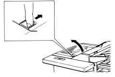
**5** Gently close the printer cover, pressing firmly on both sides of the printer cover until you hear it click.
